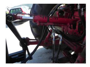
The Wintex MCL3T must be mounted on the tractor by means of a hydraulic cylinder with top link. The hydraulic hoses must be mounted on the top link.
