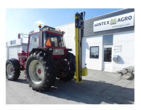
It is necessary to make a frame or another assembly so that the mast can rest against the driver's cab during transportation.
