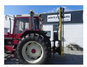
Before dismounting the Wintex MCL3T the probe must be dismounted. To avoid tipping over make sure that the drilling head is down.
