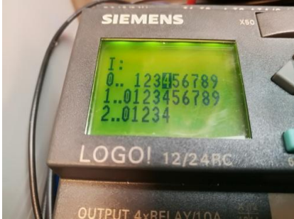
Fig. 5 The inner sensor (I4) is activated.
