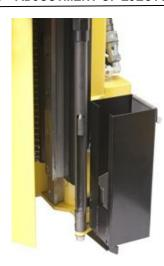
When adjusting the ejector make sure to stop the probe approximately 10 cm from the start position. Turn off the WINTEX 1000, and activate the emergency stop.
