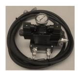
The oil pressure is pre-set at a lower limit of 50 bar and an upper limit of 80 bar. Adjusting the excess pressure valve can alter the pressure.
