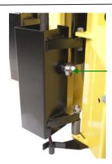
Adjust the soil box so that it is perpendicular with the soil sampler and so that the drilling head can pass.
