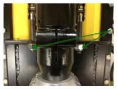
Lubricate the grease nipples.
