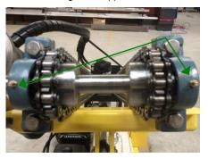
It is important to lubricate the chain with oil.
