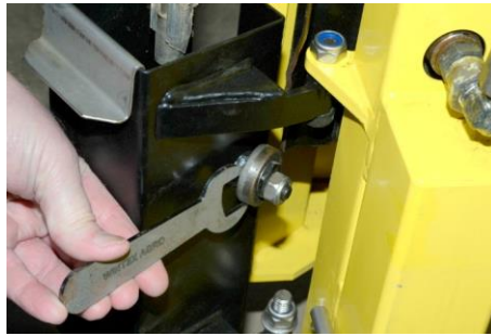
Cam Adjustment, widest part at top
