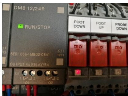
Fig. 3 The relay lights up red when it is activated.
