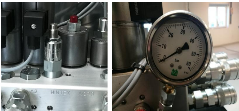
Fig. 9 The hammer adjusting valve and the gauge to read the pressure of the probe when it goes down; note that you can only read the pressure while the hammer moves downward.
