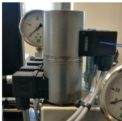
Fig. 4 The coils and connectors for the valves
