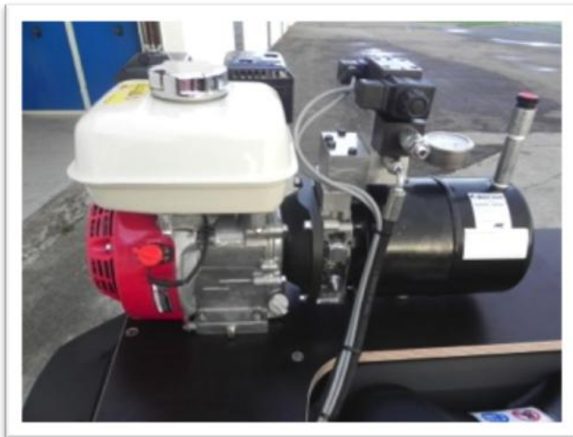
Oil pump and Honda GX 160 motor on a Honda TRX 680
